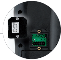
External removable EEPROM SIM module
